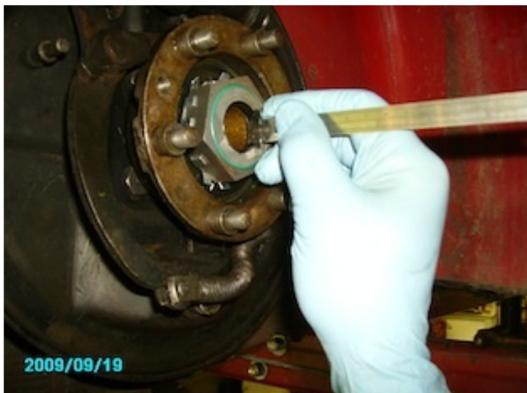
Measuring depth of seal
