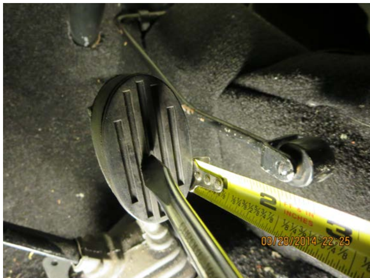
Measuring Free Travel of the Brake Pedal
