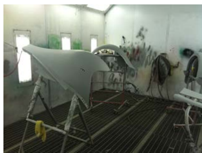
Repaired Fenders in Primer
