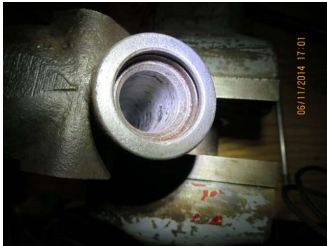
Master Cylinder Inside after Honing
