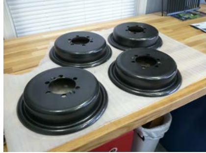
Powder Coated Brake Drums
