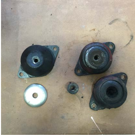
New vs Old "Squished" Engine Mounts
