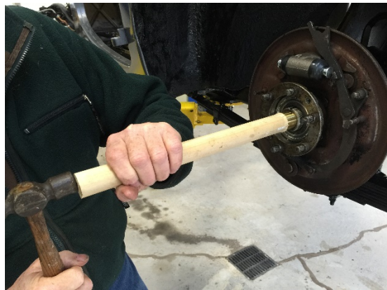
Installing New Left Rear Shaft Bushing
