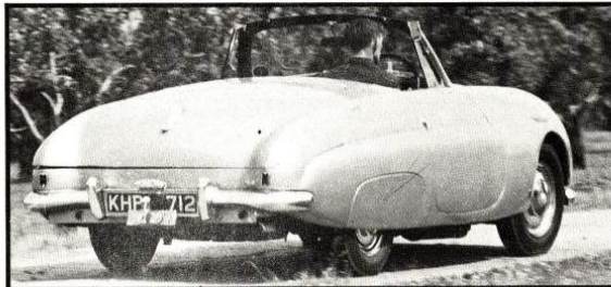
The tails of both the Bullet (left) and the Fury (right) are flat and wide – but there the resemblance ends. Note the minute brake cum tail lights of the Bullet
