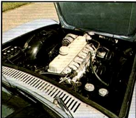
Rocker box cover spotters will instantly recognise Triumph's in-line six which nestles beneath the Fury's forward hinged bonnet (top) while that below is unmistakably vintage Vanguard
