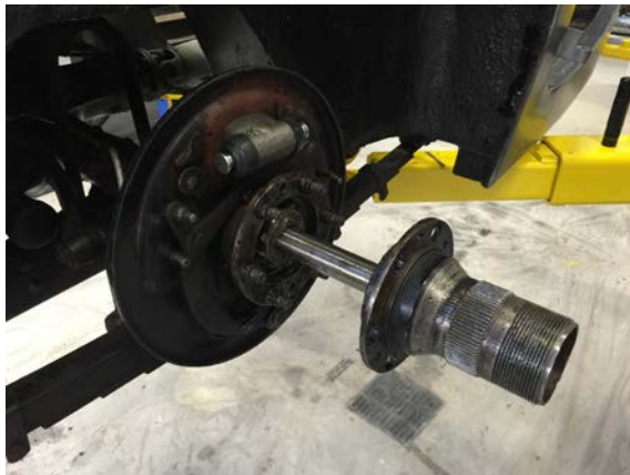
Pulling the Left Rear Hub
