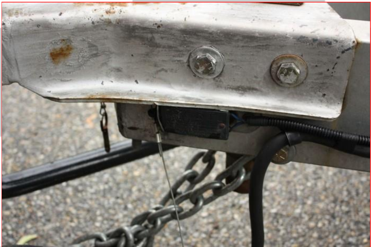
Emergency trailer brake controller; should the cable pull tight, the trailer's electric brakes activate.
