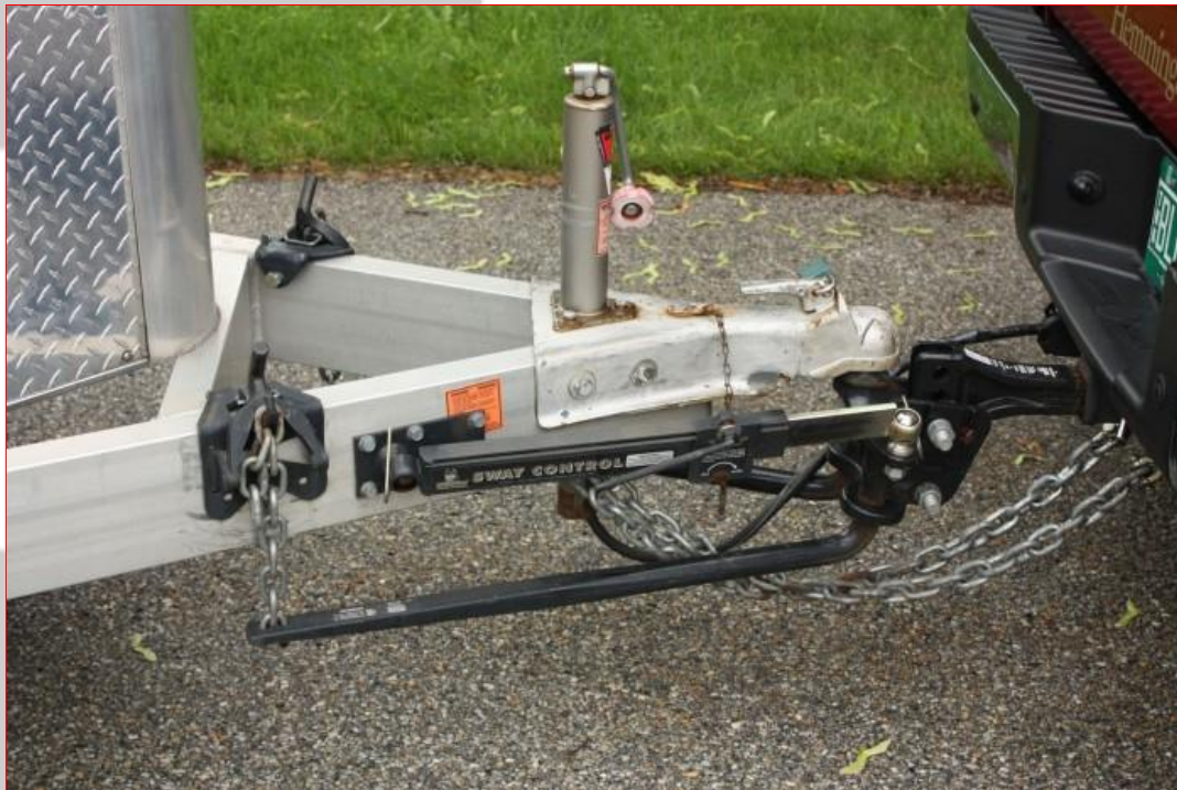
Properly hitched trailer, showing sway control bar.
