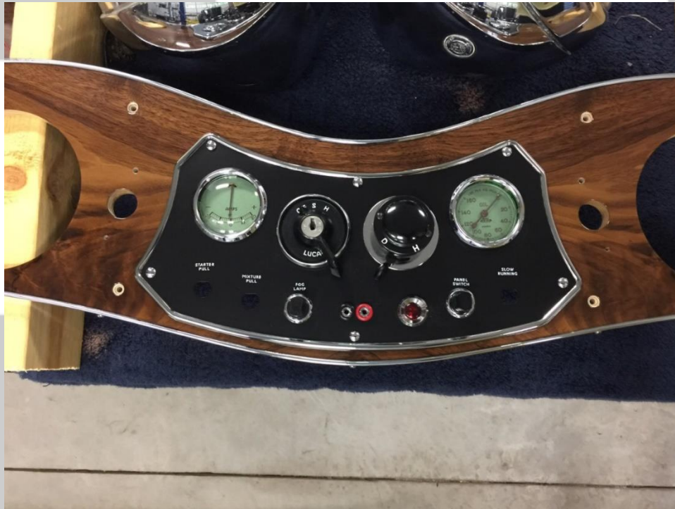
New Dashboard with Chrome Trim Installed and Renewed Control Panel
