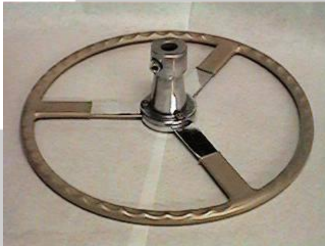
Rear of the Export gold pearl wheel with 14 finger indents per segment
